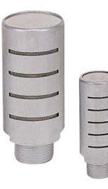
HFMA-Series high flow muffler features a 50 mesh, self-cleaning stainless steel screen and combined with corrosion-resistant aluminum shell to create a highly efficient, ultra-quiet muffler designed with minimal back pressure.
