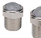
SBN-Series breather vents combines low profile and air flow into a reality suitable for many applications, particularly where space is limited. Special screen filiter is fromed by stainless steel wire, offers very high mechanical resistance, guaranteeing long life even under high pressure. Nickel plated brass fitting offers additional corrosion resistance.
