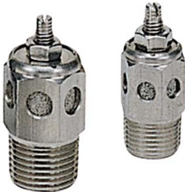
SSSCM-Series Stainless steel muffler with speed control provides infinite variation of control of airflow at an acceptable sound level on the exhaust ports of air valves or single acting cylinder with complete safety. They are constructed with 300-Series stainless steel materials, therefore they are resistant to atmospheric corrosion, foodstuffs, sterilizing solutions, many organic chemicals, dyestuffs and wide variety of inorganic chemicals.
